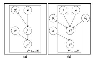
Figure 1: Graphical model for (a) m single-task Gaussian processes with m sets of: inputs  $X^i$ , temporal covariance hyperparameters  $\theta^i_t$ , estimated functions  $f^i$ , noise terms  $\sigma^i$ , and outcomes  $y^i$ ; and (b) a multi-task Gaussian process which relates m tasks through all prior variables, with the tasks' labels l and similarity matrix  $\theta_c$ .
